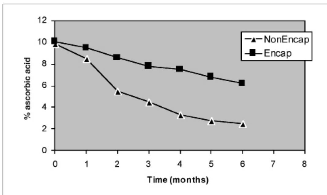
**Figure 17.7.** The stability at 45°C of encapsulated ascorbic acid versus non-encapsulated material. Note: assay for ascorbic acid was by HPLC.
