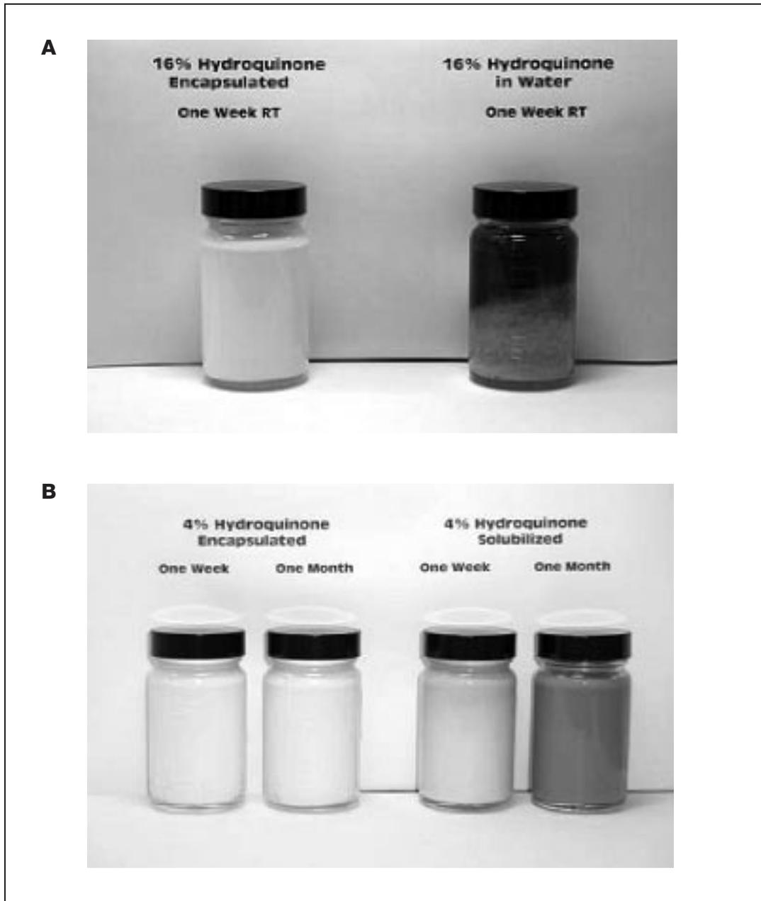
**Figure 17.8a.** Color fastness of encapsulated hydroquinone. Note: the sedimentation of the non-encapsulated hydroquinone and the dark color of the supernatant.
