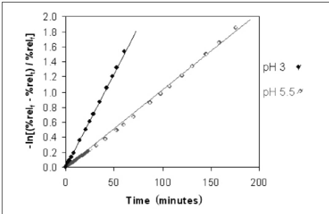
Figure 17.4. pH dependent release kinetics from a PVPy microcapsule
