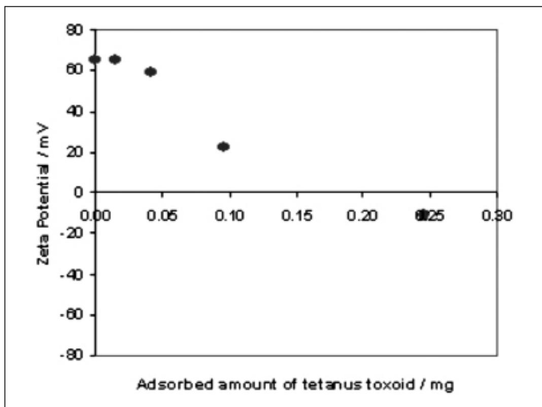
**Figure 17.12.** Effect of adsorption of tetanus toxoid on the zeta potential of a cationic SLN
