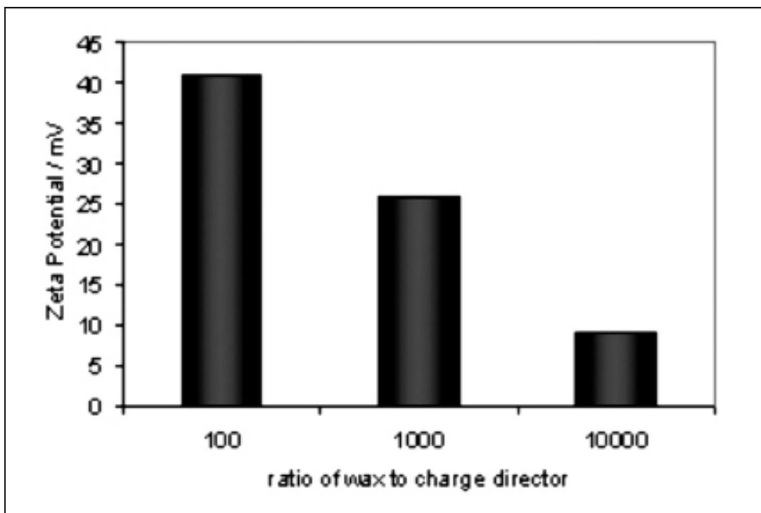
*Figure 17.13. Effect of wax: CMD ratio on the nanoparticle zeta potential.*
