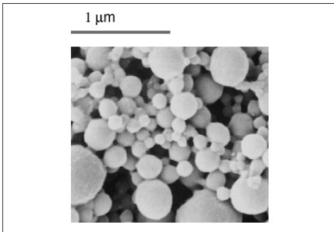
**Figure 17.6.** SEM of a typical SLN. Note that the particles are spherical but polydisperse.
