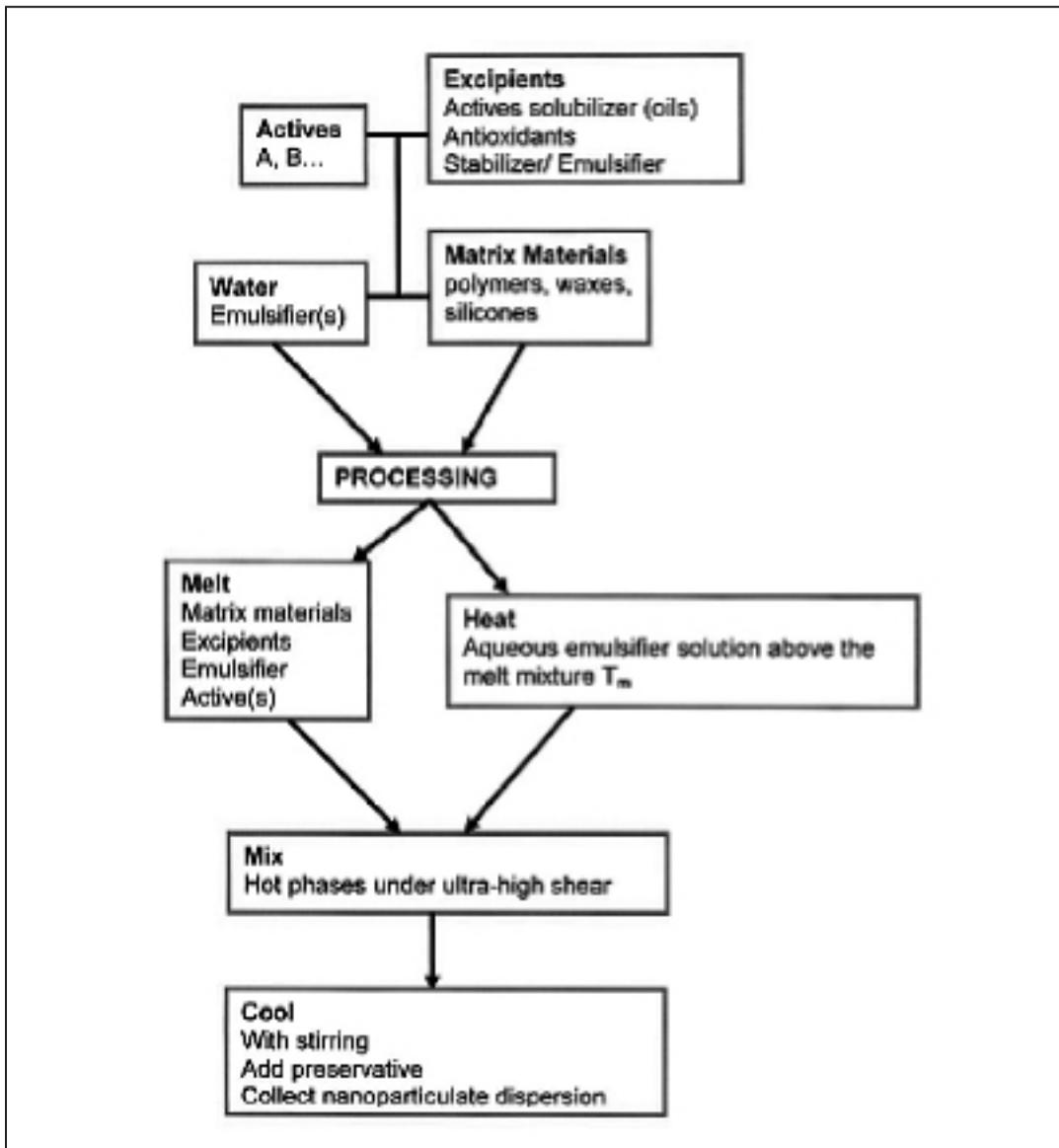
**Figure 17.5.** Schematic of the Melt-Emulsify-Chill process.
