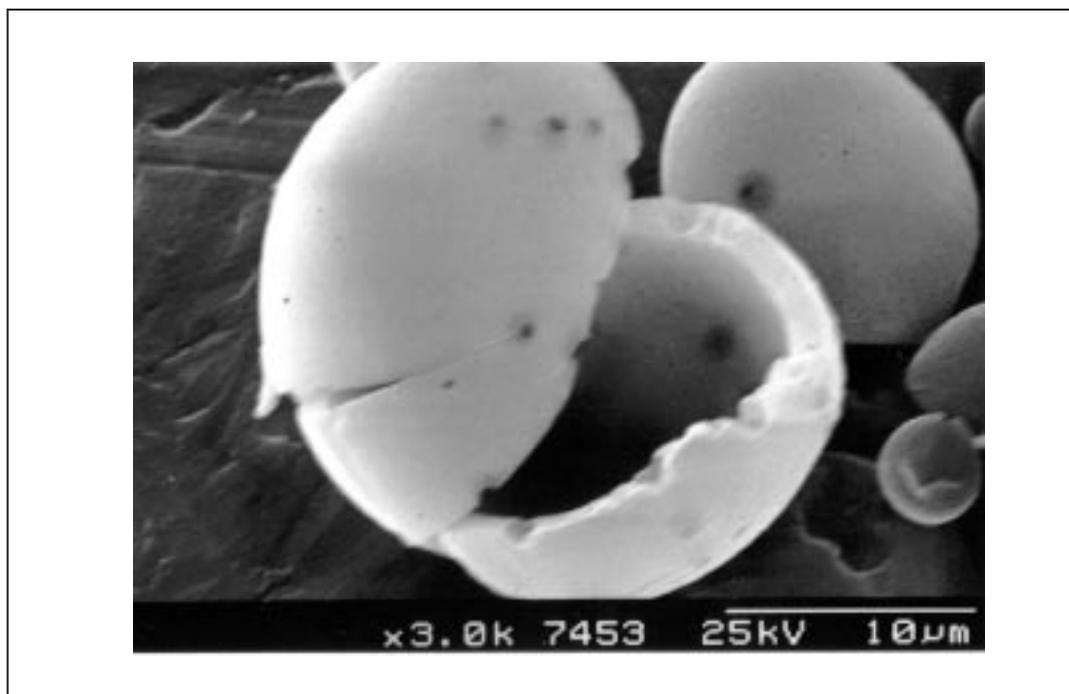
**Figure 17.3.** SEM of fractured poly(4-vinylpyridine) microcapsule.
