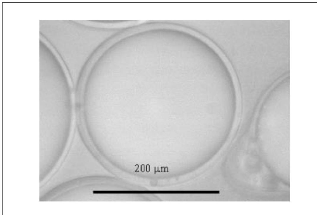
**Figure 17.2.** Optical micrograph of gelatin-acacia microcapsule prepared by coacervation.
