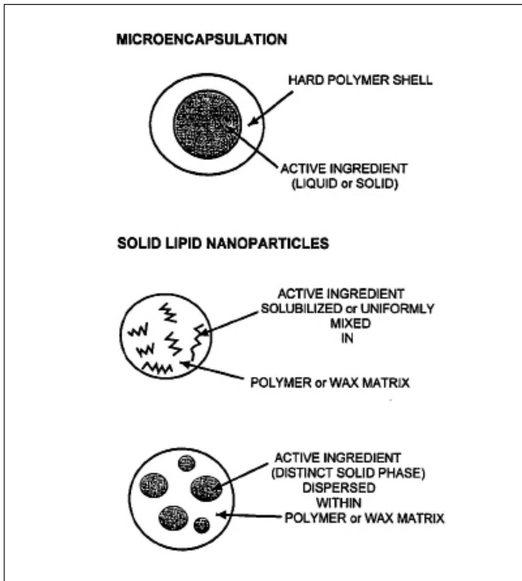
*Figure 17.1. Schematic comparing microcapsules with SLNs.*
